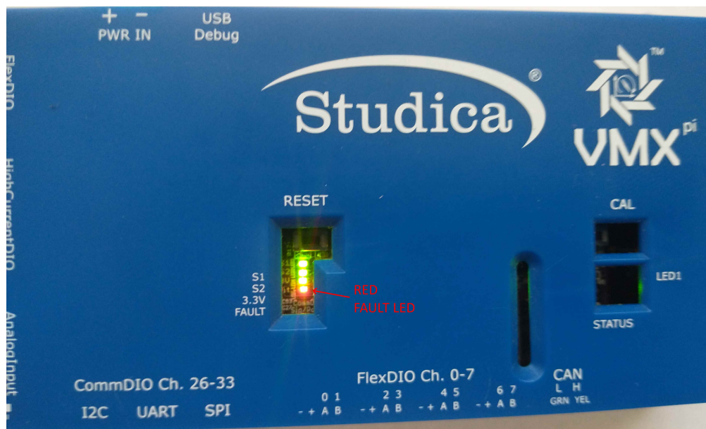
Fig. 3: VMX Red Fault LED (Overcurrent or Short Circuit Detected)
