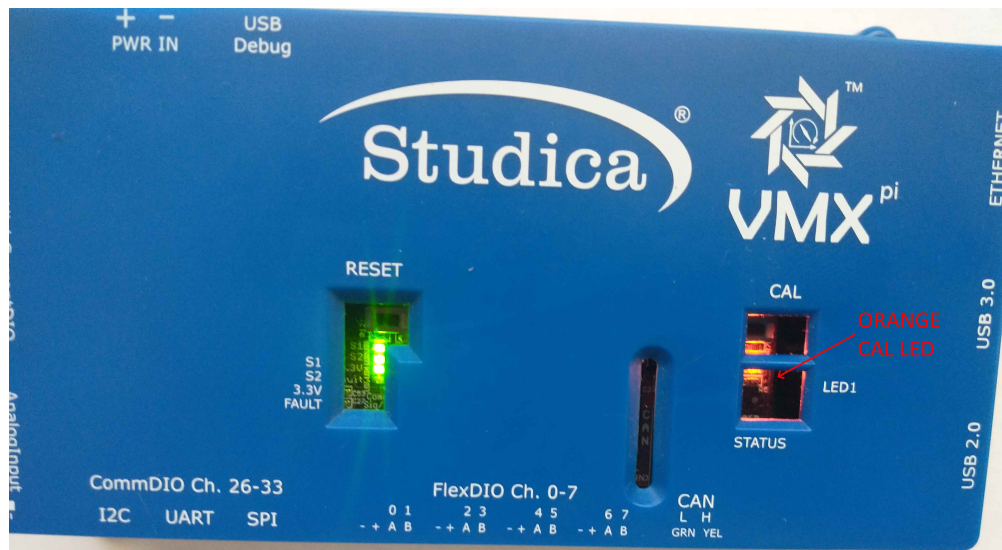
Fig. 2: VMX Orange CAL LED (navX-Sensor Factory Calibration in Progress)
