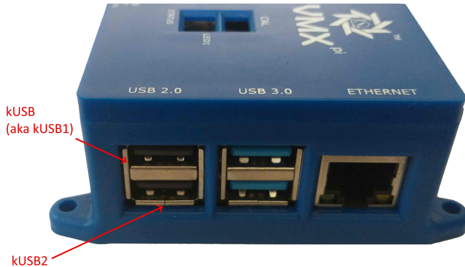
Fig. 8: Raspberry Pi USB Port WPI Library Serial Port Addressing
